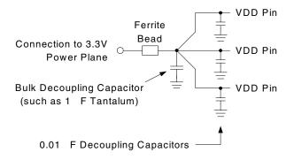
All power supply pins must be connected to the same voltage, except VDDR and VDDO may be connected to a lower voltage in order to change the output level. If the reference output is not used, ground VDDR.
