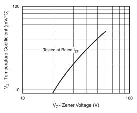
Fig. 4 - Typical Temperature Coefficients
