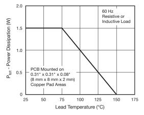
Fig. 1 - Maximum Continuous Power Dissipation
